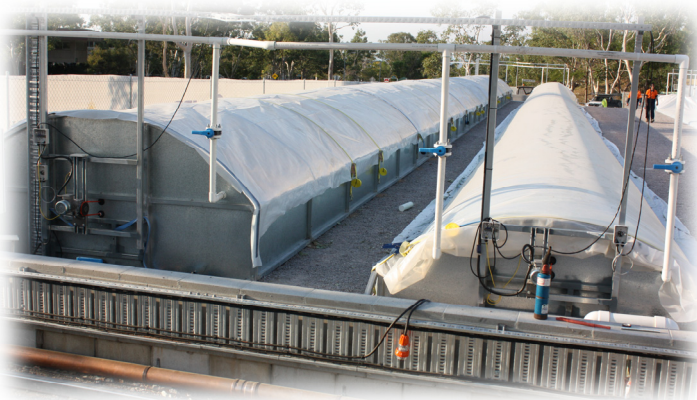
Algae under cultivation at MBD's R&D Facility. In addition to the covered units (pictured), 10 and 50 metre fully enclosed plastic membranes are also used.
